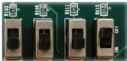
Figure 4. Slide switches connections from Spartan3FPGA Lab Kit
