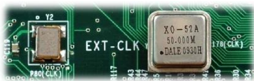
Figure 19. Clock source connections from Spartan3eE FPGA Lab Kit
