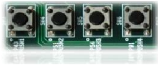
Figure 6. Push Button interface from Spartan3 FPGA Kit
