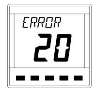
In the unlikely event that your Network NAV unit should develop an internal error, the unit will sound its alarm continuously and the display will show an error number. Pressing the keys will not silence this alarm.
