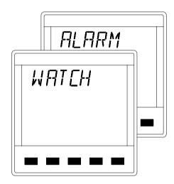
The Watch Alarm is a count-down timer which is activated at the end of the preset count-down period. The display alternates between the messages above.
