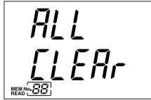
ALL CLEAR alarm indication
