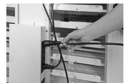
**Step 5:** Starting with the top IEC lead plug the connector in to the laptops power pack.
