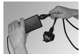
**Step 3:** All **LAP16H** models are supplied with 16 x IEC to figure of eight & 16 x IEC to cloverleaf cables to be connected into the laptop power pack & the IEC power strips. Firstly select the leads with corresponding connector for the power packs being used in the cart.
