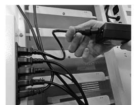
**Step 6:** Then place the power pack onto the rear storage area of the top shelf and push the laptops connecting lead through to the front of the shelf. Repeat until all power packs and leads are in place.
