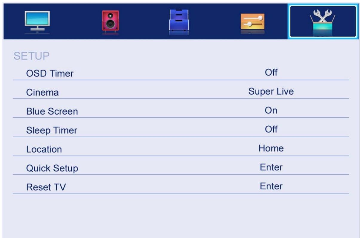
1. Press ▲/▼ button to select the option that you want to adjust in the **Setup** menu, then press **ENTER** or ▶ button to enter.
