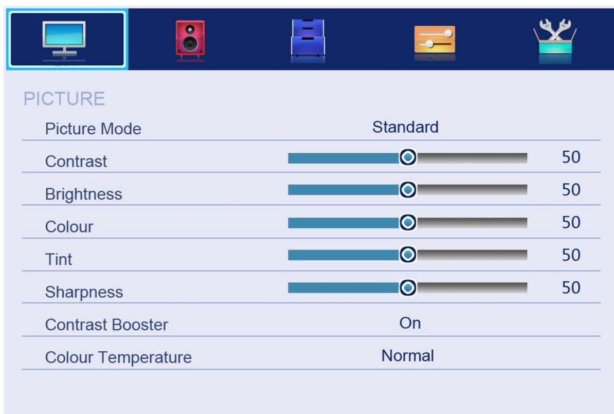
1. Press **▲/▼** button to select the option that you want to adjust in the Picture menu, and then press **ENTER** button or **▶** button to enter.
