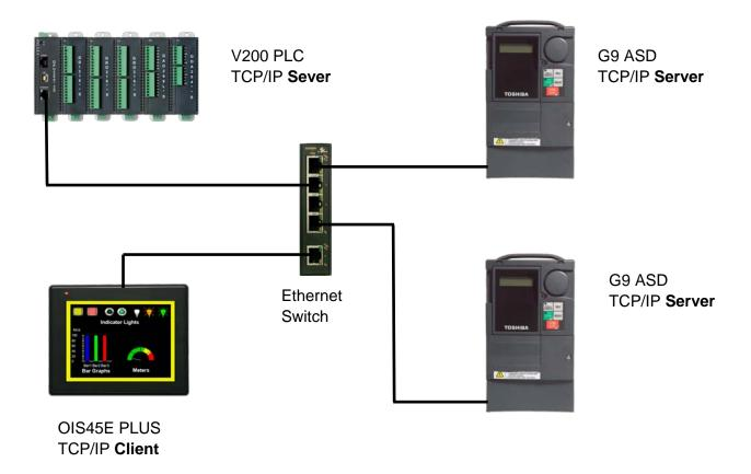
For the Ethernet Modbus TCP/IP network example, just one client and one server will be used. The objective is to show the setup and verify the communications.
