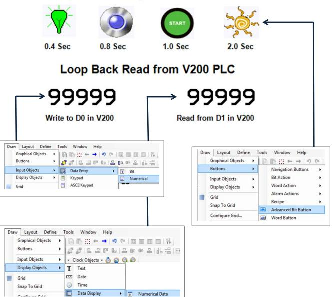
Now the tags can be attached to the screen objects. Often times it is easier to attach the tags to the objects as the objects are created. It can be done either way.
