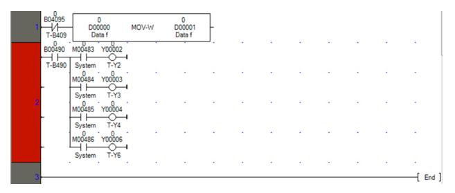
Note: Programming outputs Y00002 thru Y00006 is not necessary. But it does allow confirmation of the special M timing bits in the V200 PLC. These are the same timing bits that control the bit buttons on the OIS45E PLUS.
