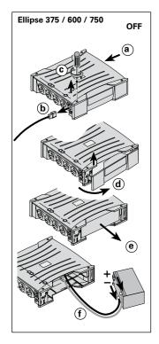
Warning: take care not to inverse the polarity + (red) and - (black) when connecting the batteries as this will destroy the device.
