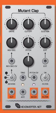
The NOISE output is a voltage controlled C64-like noise oscillator! You can use it just like a VCO in your system.
