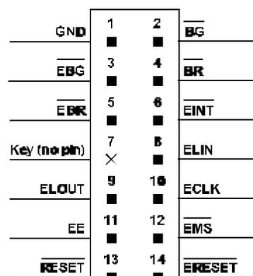
Figure 2a. Target board emulation header
