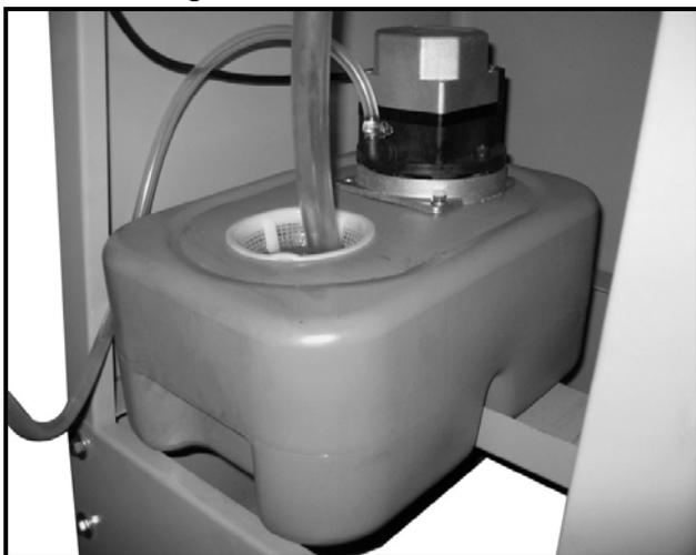
Figure-12 Coolant tank inside the stand
