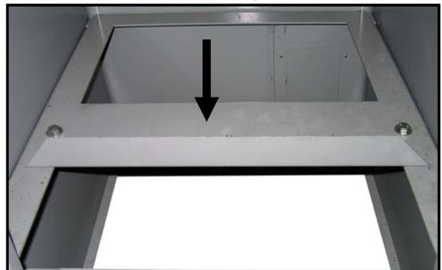
Figure-4 Installing the coolant tank bracket
