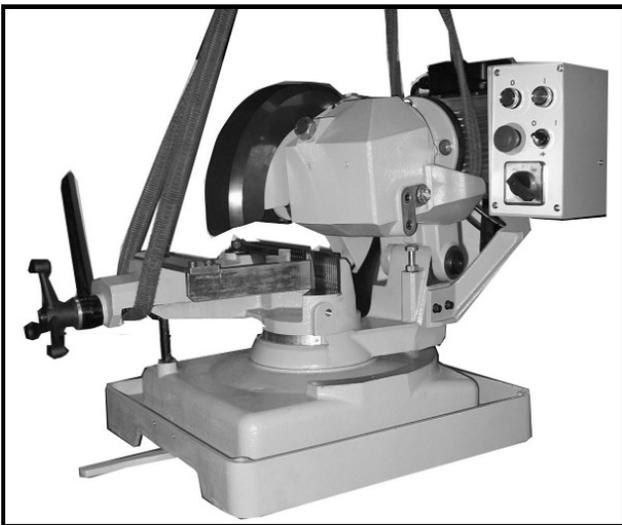
Figure-2 Lifting straps around the motor and the jaw of the CX110
