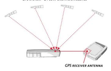
The number of satellites in view and reception strength of each GPS satellite will govern how long time the terminal will use to to get a fix. Typical fix times are between a few seconds to 5 minutes. However, as a minimum of 3 satellites is required to get a fix at all, there will exist positions and times during the day, where the terminal will use longer, or in worst case will not get a fix at all.
