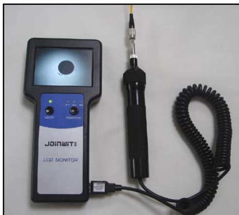
Probe with handheld monitor
