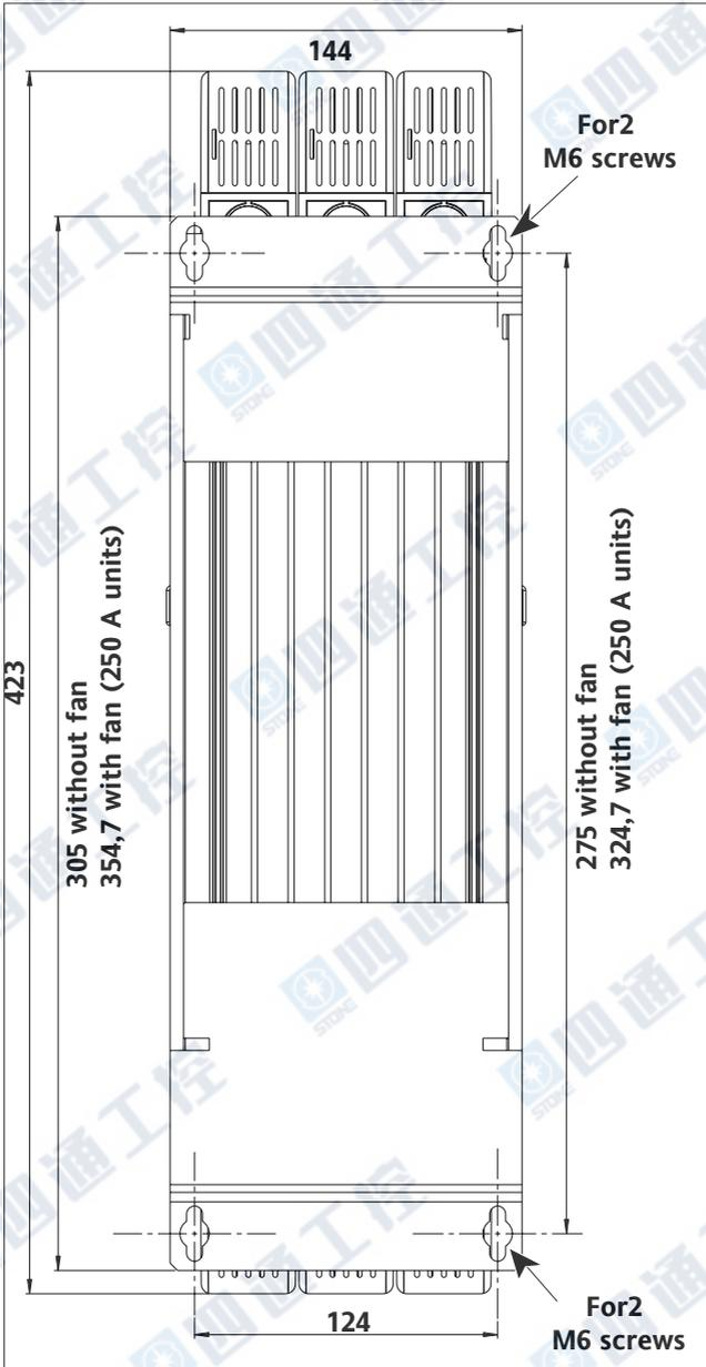
Figure 2-5 125A to 250A 7100 A unit mounting
