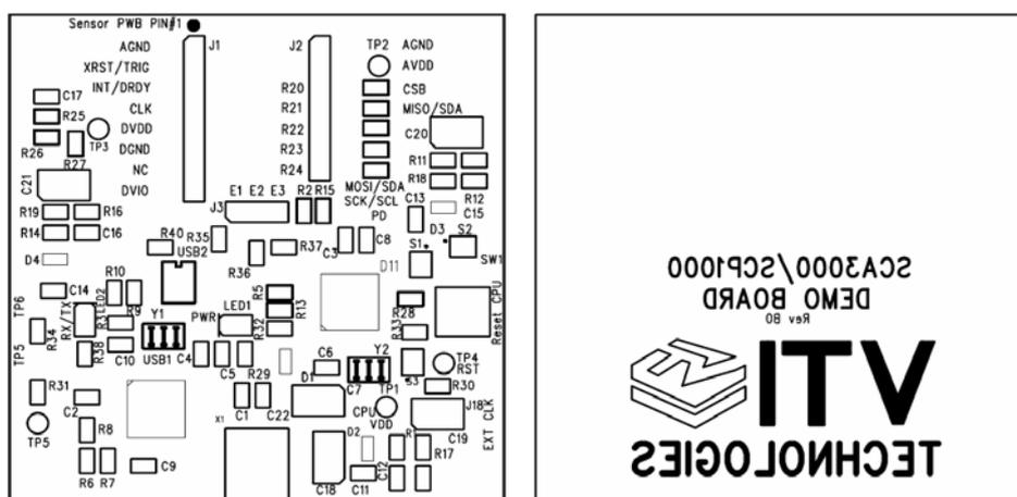
Figure 15. SCC1300 Demo Kit USB interface board silkscreen.
