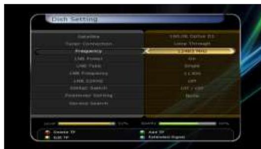
**NOTE : Tuner Connection menu is disabled if receiver is not configured with twin satellite tuners.**
