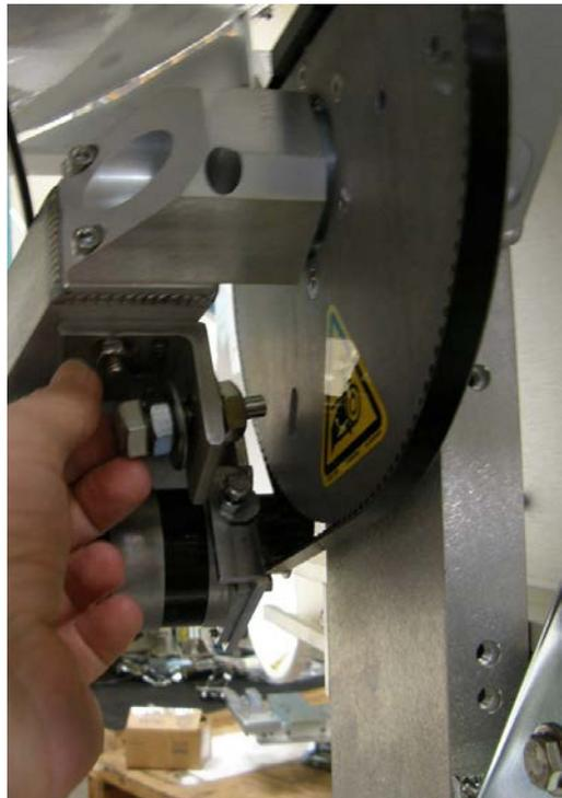
8. Tighten the hex nut to prevent the hardware from loosening while in the un-stowed configuration.
