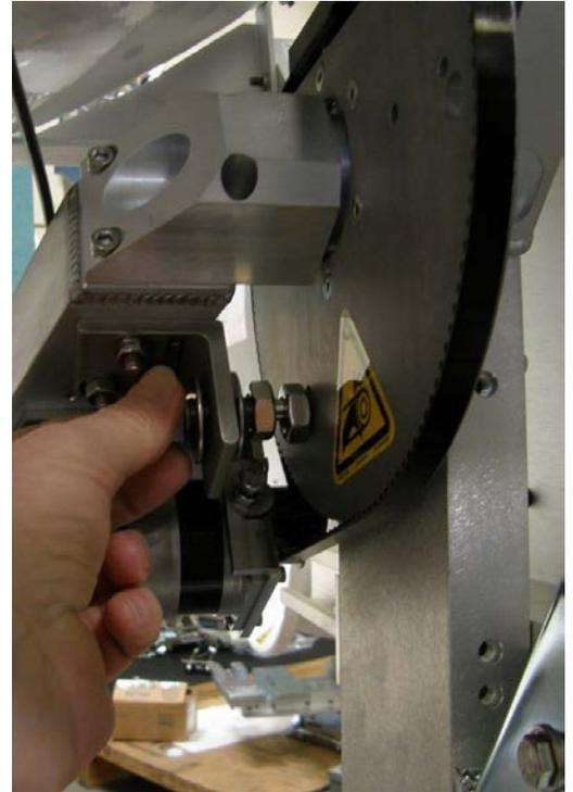
8. Tighten the hex nuts to prevent the hardware from loosening while in the stowed configuration.
