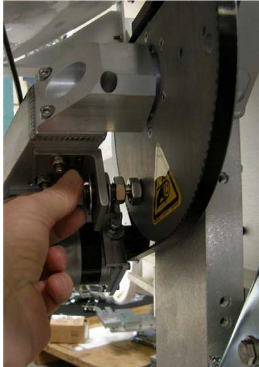
5. Remove the washer from the stow pin-bolt and thread one of the two hex nuts onto the bolt and tighten.
