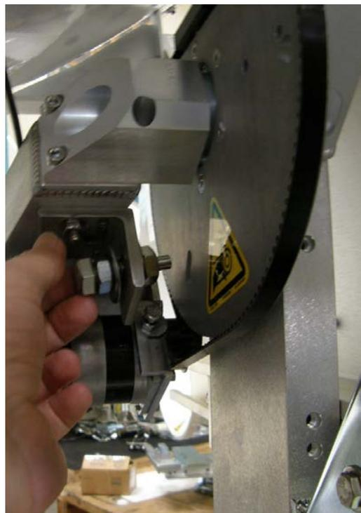
5. Remove the washer from the stow pin-bolt and unthread the hex nut from the bolt.
