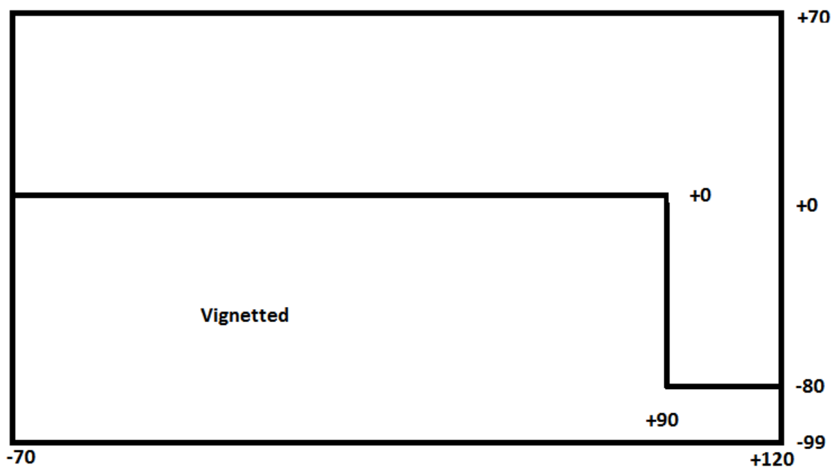
Figure 25: Blanco guider patrol area relative to the KOSMOS field of view. Selection of guide stars within the lower region can cause the guide probe to vignette the COSMOS field. The size of the region that leads to vignetting is somewhat conservative, particularly for longslit spectroscopy.
