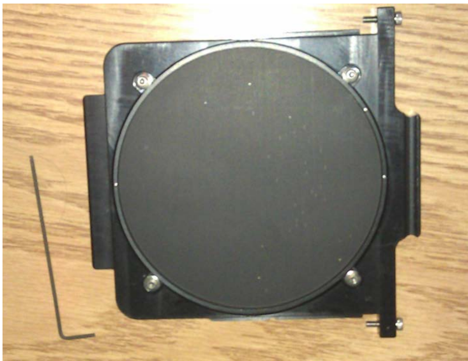
Figure 35: Mask installed in holder. Note black side facing up.
