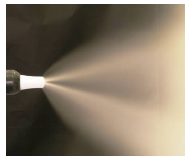
too much electrode rinsing air
