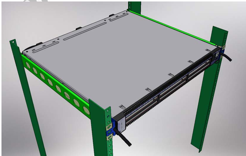
Figure 40: Transfer Power Cord Finished
