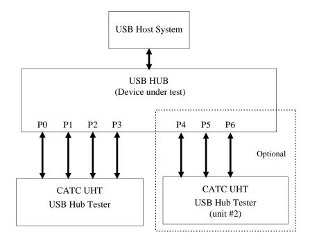
The UHT system includes a box (hardware) and a DOS application program (software) that controls the test process by communicating directly with the PC USB Host Controller.
