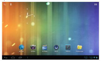
**Shutdown:** Press the power button, pop-up Power off, Click OK, you can safely shut down.
