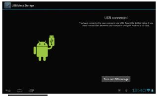
Click Turn on USB storage, Then the device can transmission data with PC.
