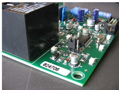
Quick Test jumper in position TEST
