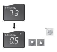
When cooler is operating, press the 'Off Timer' button and set the length of time you want by pressing ▲ or ▼. Each time you press the button you will increase the 'time to off' period by 30mins. up to 10 hours, and 1 hour thereafter up to 24 hours. The display will show .5 for 30min and 1 for an hour. e.g. One and a half hours will show 1.5.
