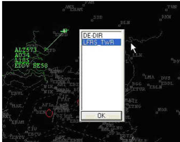
Figure 7.32 - select controller for transfer
