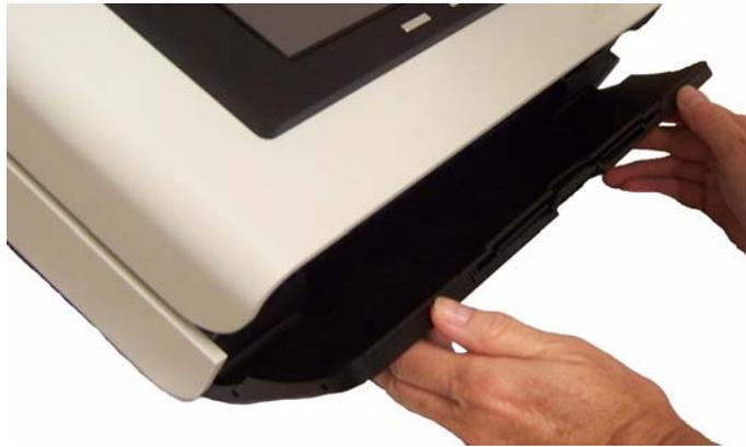
4. Adjust the output tray by pulling out the extender if needed.
