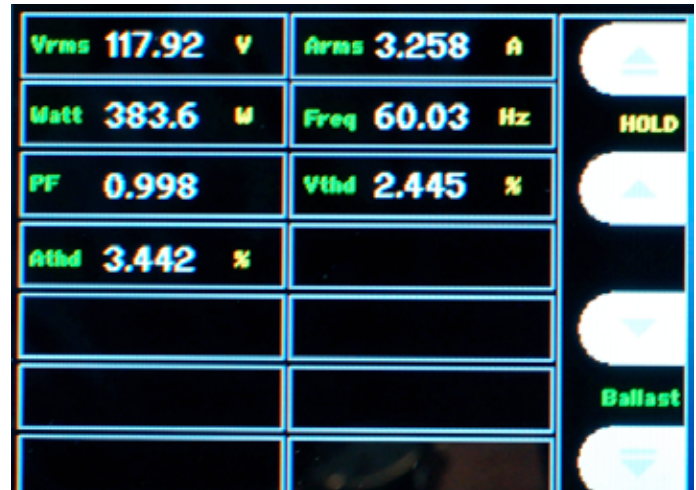
Figure 17. Example of Ballast output result display Window.
