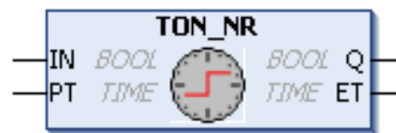
Figure 4-72. TON_NR Function Block
