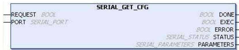
Figure 4-53. Block to Capture the Serial Configuration
