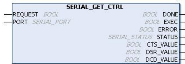
Figure 4-54. Block Used to Visualize the Control Signals
