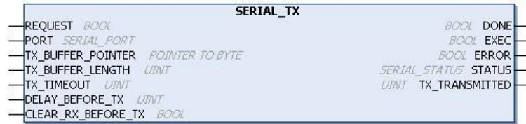
Figure 4-60. Block for Values Transmission by the Serial
