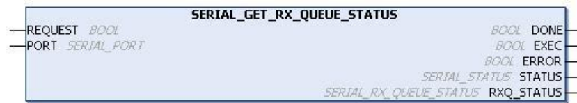
Figure 4-55. Block Used to Visualize the RX Queue Status
