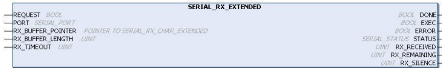
Figure 4-58. Block Used for Reception Buffer Reading
