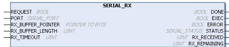
Figure 4-57. Block Used to Read the Reception Buffer Values
