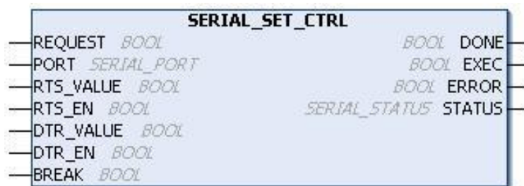
Figure 4-59. Block for Control Signals Writing
