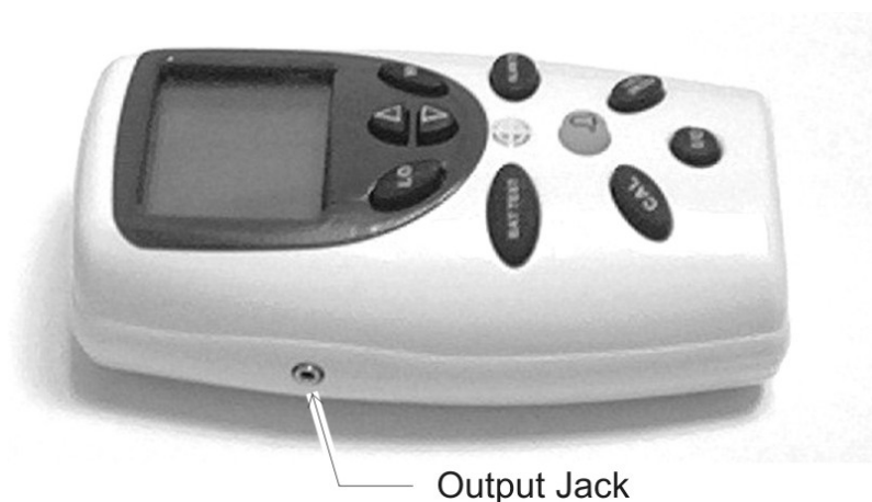
Figure 2-9: 0-1 VDC or RS 232 Digital Output Port
