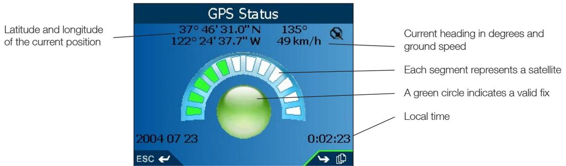
The circle under the satellite segments is green when there is a valid fix (2D or 3D), and red when there is no fix. While a 2D fix is sufficient to maintain a valid fix, a 3D fix is more accurate.
