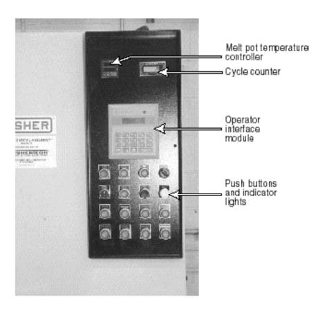
The control panel, mounted on the front of the electrical enclosure, houses
