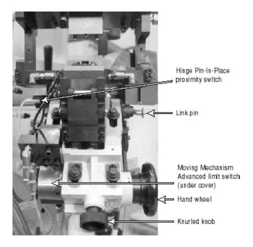
Moving mechanism and limit switch
