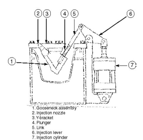
The injection unit is a piston type pump, with the gooseneck portion submerged in the alloy. The injection unit is activated by the Injection cylinder.
