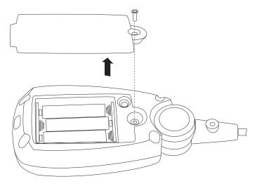
Remove the battery door to expose the three AAA batteries. Replace only with AAA batteries approved in this document. Replace the battery door and reinstall the hex screw. Be sure to use only the approved list of batteries. Any substitution will void the safety ratings of this product.
