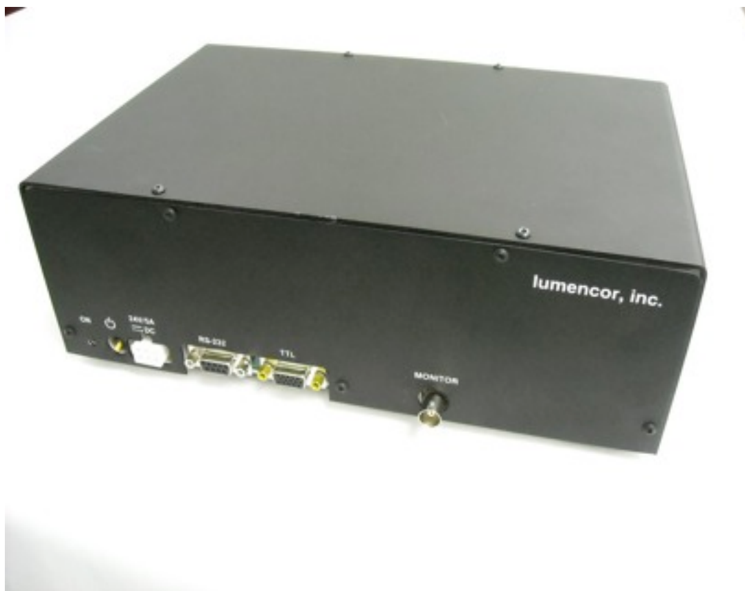
Rear Panel of SPECTRA light engine
