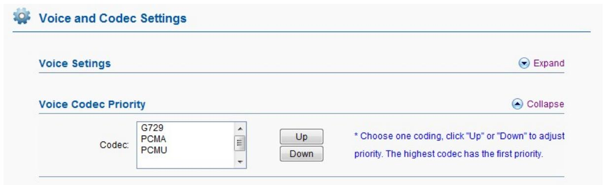
Three codec types are provided to adjust GoIP Gateway to different network environment. The top codec will be chosen to use by default. G729 uses the least bandwidth.
