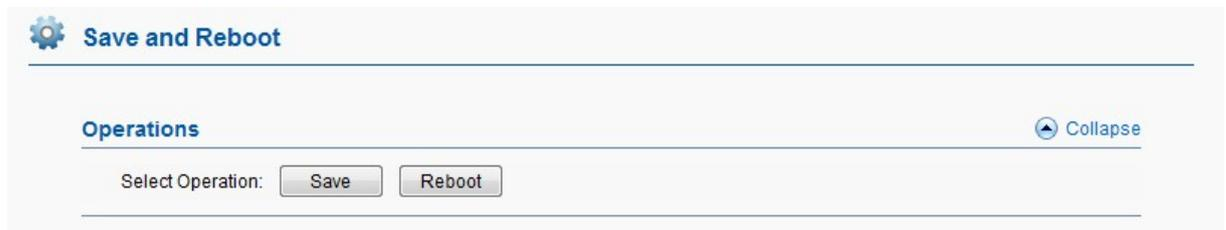
The screenshot above shows the operation buttons. Button Save is used to save all the modifications while button reboot is used to save modifications first and then reboot device immediately.
