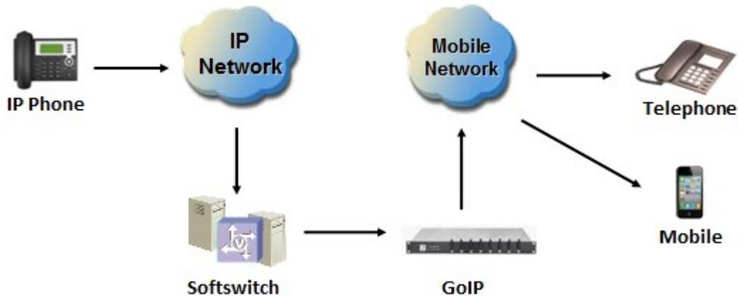
GoIP Gateway is now used more and more for telephone carriers to land their IP calls to mobile network. It plays the role of converting IP telephone signal to GSM telephone signal, relaying the media stream between IP network and Mobile network.
