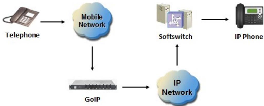
GoIP Gateway can be used as the access from mobile network to IP. Any call made to the mobile card inserted into GoIP Gateway will be routed to IP network and connected to Softswitch server. The Softswitch server can redirect the caller to final destination user.
