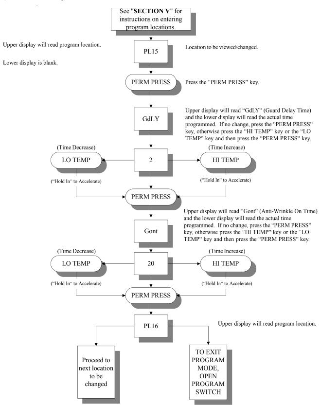
**Summary**: Guard Delay Time is programmable from 1 to 9 minutes. Guard On Time is programmable from 10 to 99 seconds.
