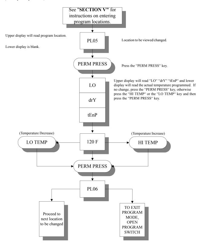
**Summary:** LO TEMP is programmable from a minimum of 110° F to a maximum of 150° F in 5° increments or from a minimum of 43° C to a maximum of 66° C in 1° increments.
