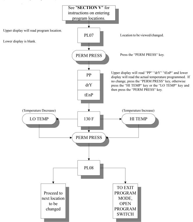
**Summary**: PERM PRESS DRY TEMP is programmable from a minimum of 110° F to a maximum of 150° F in 5° increments or from a minimum of 43° C to a maximum of 66° C in 1° increments.
