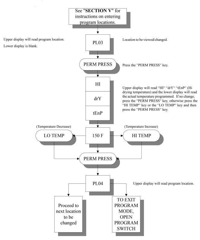
**Summary**: HI Temp is programmable from a minimum of 110° F to a maximum of 150° F in 5° increments or from a minimum of 43° C to a maximum of 66° C in 1° increments.
