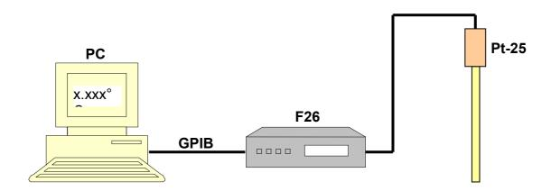
The formula for calculating temperatures is depending on two coefficients **a** and **b**. These coefficients have different values for temperatures <0.01 °C and >0.01 °C respectively.
