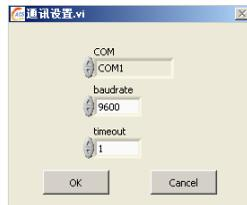
To choose the correct COM port, and set the baud rate to be 9600, then press OK to confirm, then can finish the connection between the upper computer and the mosaic controller.
