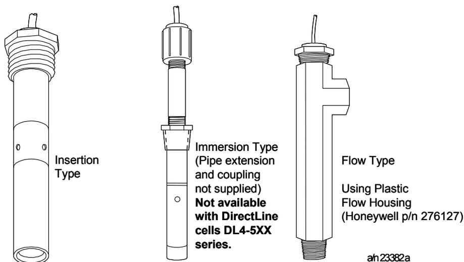
Figure 3-1 Types of Mountings for 4905 Type Cells
