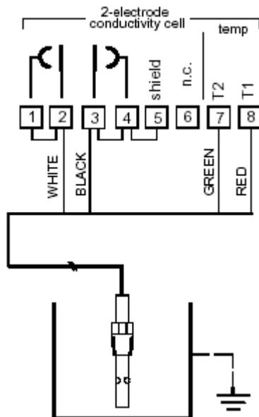
Figure 3-9 04905 series cells with or 20' leads connected to an APT2000
