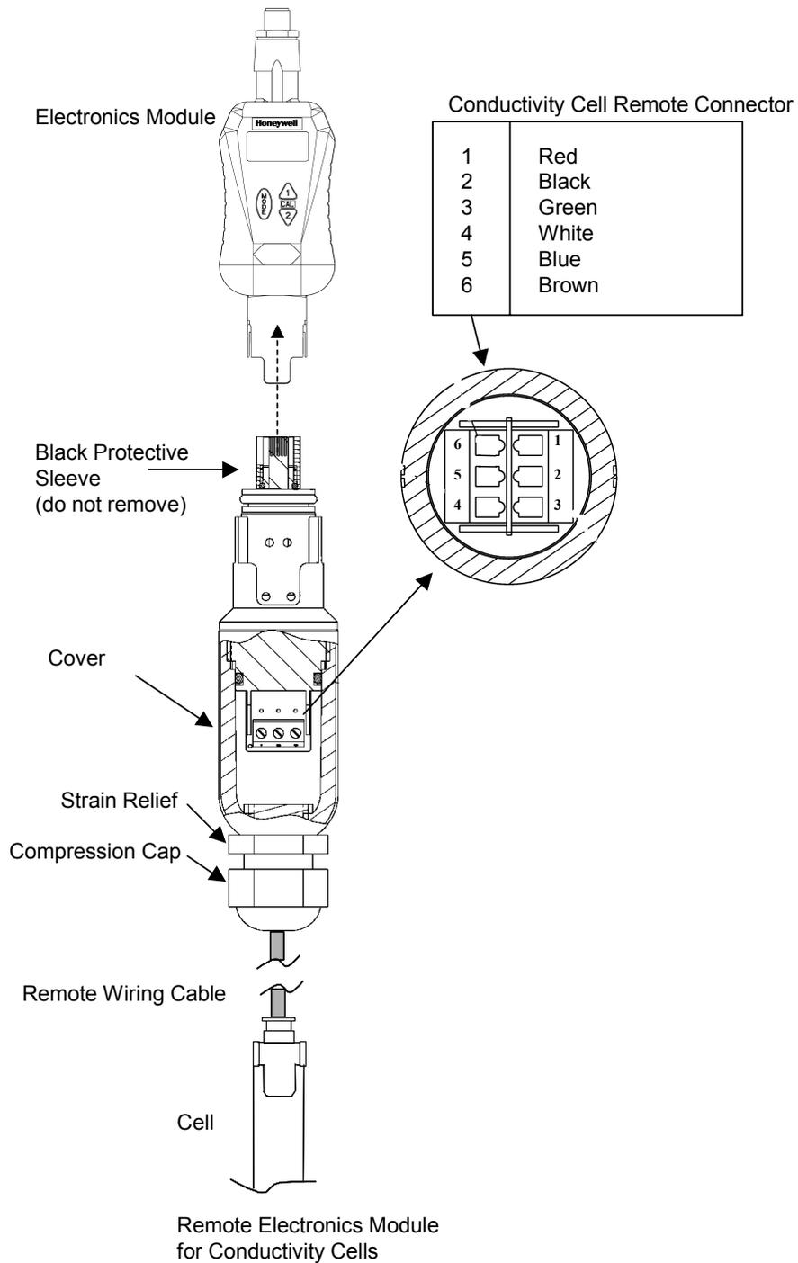
**Figure 3-11 Remote DirectLine DL4-5xx series with 20' lead connected to a DL423 Modbus (through the use of the Remote Connector Assembly)**
