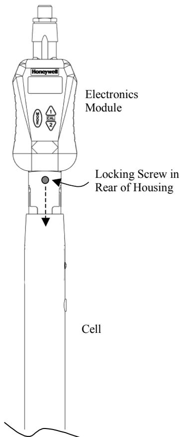
Figure 3-10 Integral DirectLine Mounting with DL4-5xx
