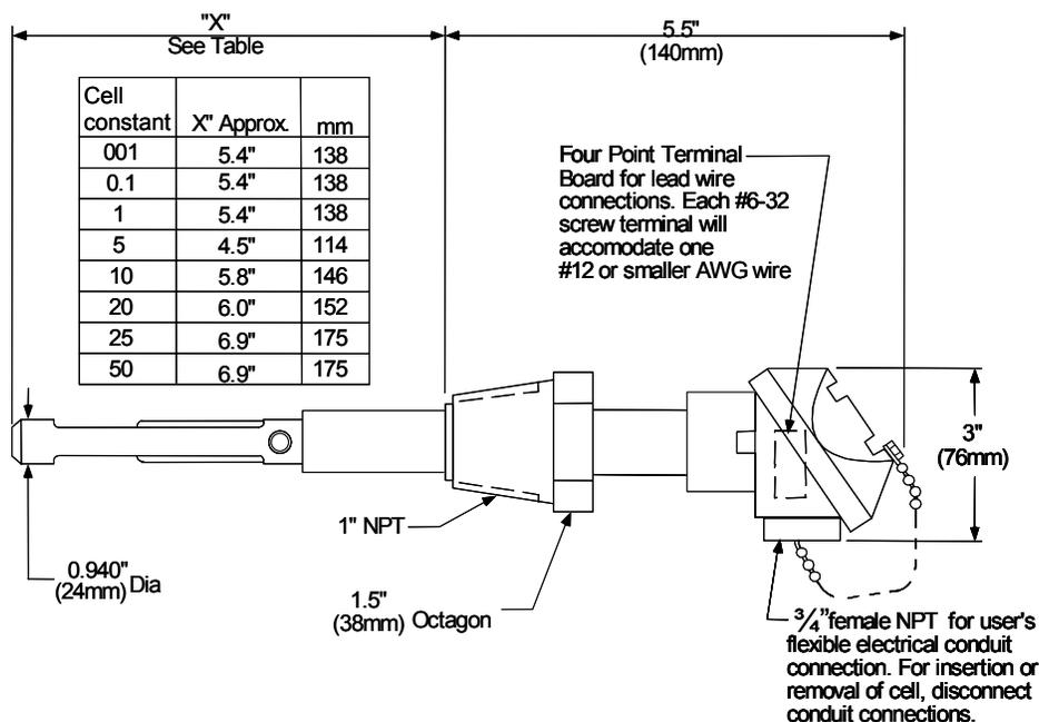
NOTE: For existing users with conduit, a 3/4" x 1/2" adapter bushing will be required to use existing conduit.
