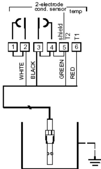
Figure 3-8 04905 series cells with 20' leads connected to an APT4000
