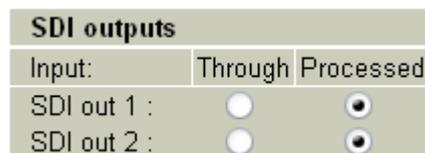
Figure 16: Multicon GYDA view of the SDI output selection block
