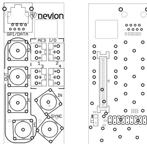
**Figure 4: FRS-HD-XMUX4-C1 backplane**
