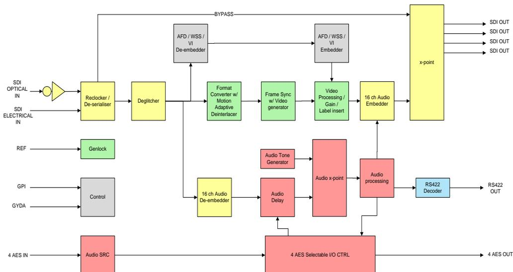
Figure 1: Simplified block diagram of the UDC-HD-XMUX4 card
