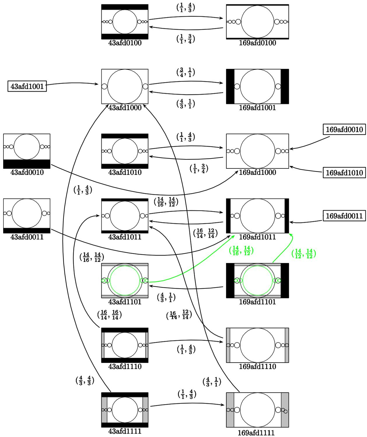
Figure 8: AFD controlled aspect ratio conversions
