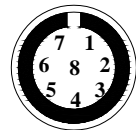
4/8 pins female Binder 712 connectors pinout: external view
