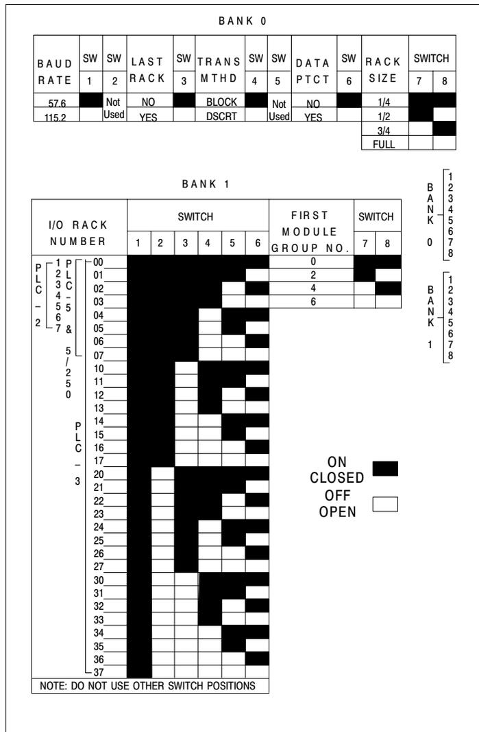
Each switch bank has eight switches. Set each switch to the ON (closed) position by depressing the right-hand side of the switch or to the OFF (open) position by depressing the left-hand side of the switch (Figure 3.2).
