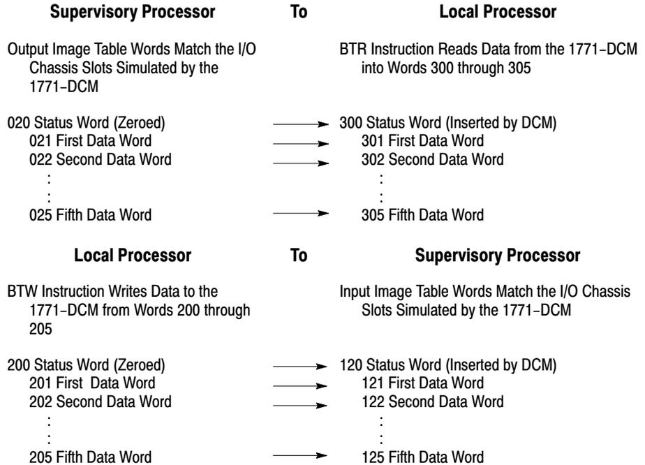
Your ladder program for the supervisory processor must place data in output image table word addresses for transfer to the 1771-DCM and move data from input image table word addresses as needed by your application. We leave this ladder logic to you because your application and processor's set of instructions determine how you would do this.
