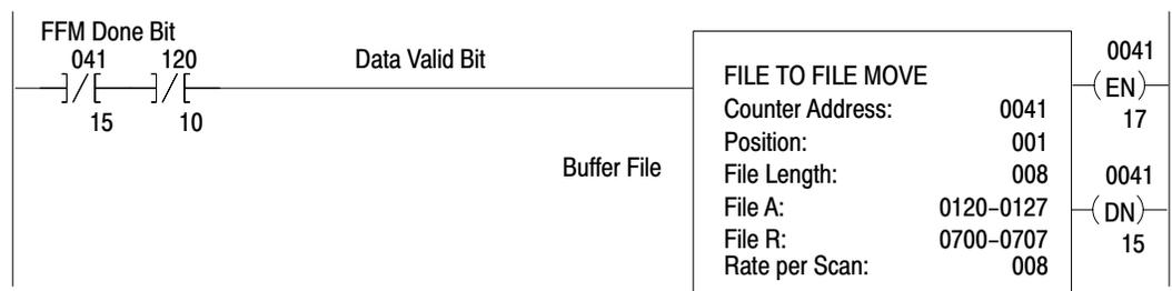
Your ladder program must place data into output image table words for transfer to the 1771-DCM. Avoid placing data in the first word because the 1771-DCM inserts status in this word. We leave this ladder logic to you because your application and processor’s set of instructions determine how you would do this.
