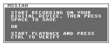
The procedure for saving and loading SDR data is very simple. You are asked to start your digital device and then press space to start the C64 read/write sequence. Saving can be switched to verifying instead. That makes the program read from the SDR device comparing the saved data to the current memory. The save is then considered valid if the SDR data is identical to the memory data.
