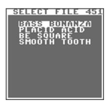
The file operations for the floppy drive make use of the operating system's basic disk functionality. There are no delete-functions and no replace-and-save options built in. If you try to save the file onto disk using an already existing name the save is interrupted and the drive light flashes.
