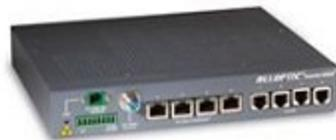
This device will be installed internally to your home if you have a Fibre to the Home (FTTH) based solution. If your estate has a Fibre to the Curb (FTTC) installation this device will be installed a street kiosk and shared by 4 houses
