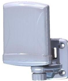
This device will be externally mounted on your house if you have a wireless Access method for service delivery from the estate network to your house. Please note that this device is not used for wireless internal home networking. It is only a service delivery access point onto the ATEC internal network
