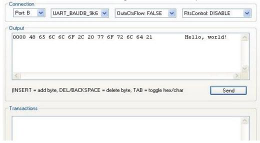
Clicking on "send" button will send "Hello, world!" on the serial channel. If HyperTerminal has been set to the correct communication speed, the same message will be displayed on the screen.
