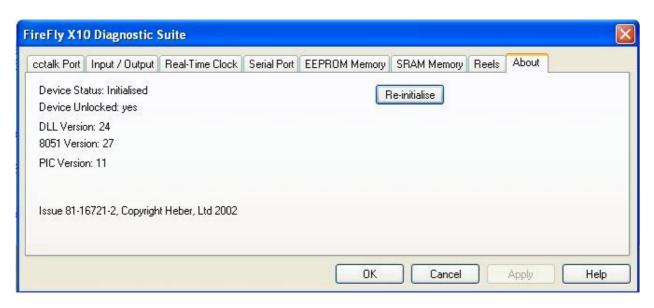
At anytime while running the program, if USB connection is lost, clicking "Re-initialise" should restore the USB connection between the firefly X10 board and Windows operating system.
