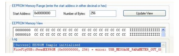
When setting a correct start address and a correct number of bytes to read which will not exceed the memory range (EEPROM = 512 bytes --- Can be accessed from 0x8 to 0x1FF → last byte to be written is 0x1FE) the memory view will be displayed as follow when clicking "Update View" button and no message will be displayed in the "Log" part.
