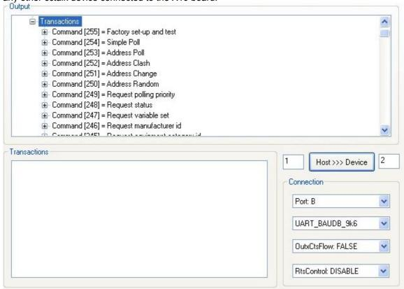
When selecting a command from the output window and clicking "Host>>>Device" button, the corresponding line of the XML script is executed.
