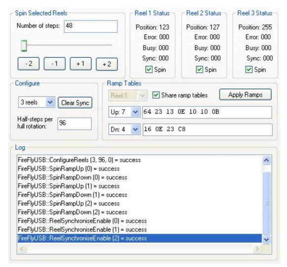
The status of the reels is displayed in the top right corner of the window. The position is set to a random position and will be used as a reference later in order to display the new position according to how far the reel spins. It does not update from the optical index sensor on the reel). When spinning all the reels, a specific reel can be disabled or enabled by changing the "Spin" check box.
