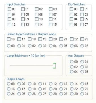
The first time the "input/output" tab is clicked, the program reinitializes all the output lamps to 0 (no light) and updates all the inputs to the status of the switches on the board.<sup>1</sup>
