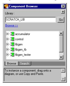
From the Component Browser select the *fibgen* component, hold down the left mouse button and drag the component onto the block diagram. Repeat this procedure for the *fibgen\_tester* component. The diagram should look similar to the one shown below:
