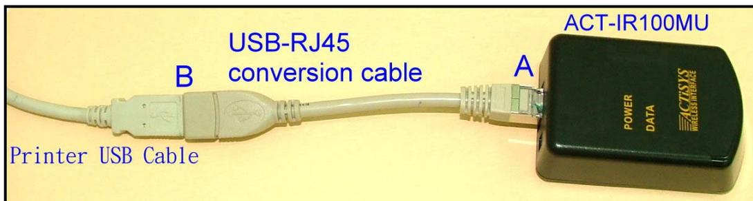
**Step4:** Connect printer USB cable from printer to USB-RJ45 conversion cable as shown at above point B
