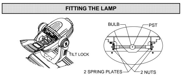
Lock tilt before fitting/replacing the lamp.
