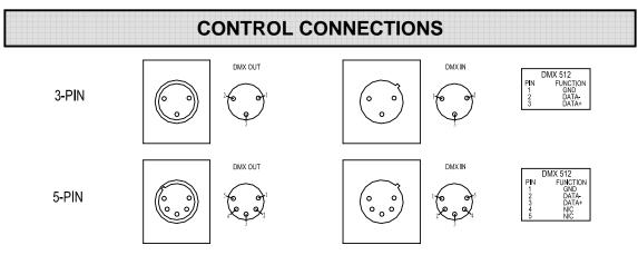
Connection between controller and projector and between one projector and another must be made with 2 core-screened cables, with each core having at least a 0.5mm diameter. Connection to and from the projector is via cannon 3 pin (which are included with the projector) or 5 pin XLR plugs and sockets. The XLR's are connected as shown in the figure above.
