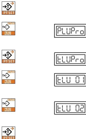
1. In normal working mode, place the tare weight on the platform and press
