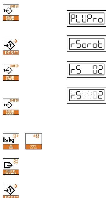
1. Keep pressed the key for longer than 1 second to access the User's Programming.
