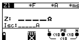
Figure 5.30: Line impedance measurement menu
