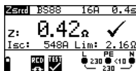
Figure 5.29: Example of fault loop impedance measurement results using trip-lock function
