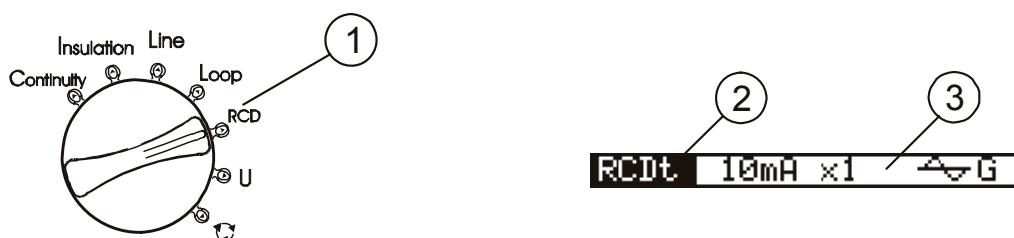
Figure 4.2: Function selector switch and belonging parameter line
