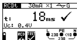
Figure 5.15: Example of trip-out time measurement results
