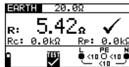
Figure 5.41: Example of resistance to earth measurement results
