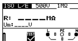
Figure 5.1: Insulation resistance measurement menu
