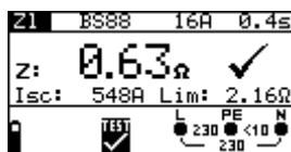
Figure 5.32: Example of line impedance measurement results
