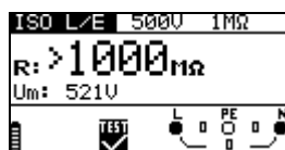
Figure 5.3: Example of insulation resistance measurement results
