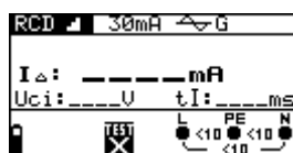
Figure 5.16: Trip-out current measurement menu
