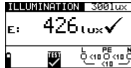
Figure 5.47: Example of illumination measurement result
