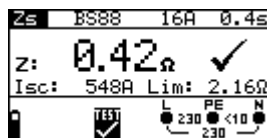
Figure 5.27: Example of loop impedance measurement results
