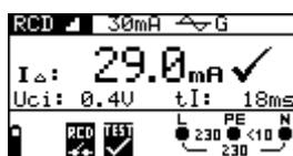
Figure 5.17: Example of trip-out current measurement result
