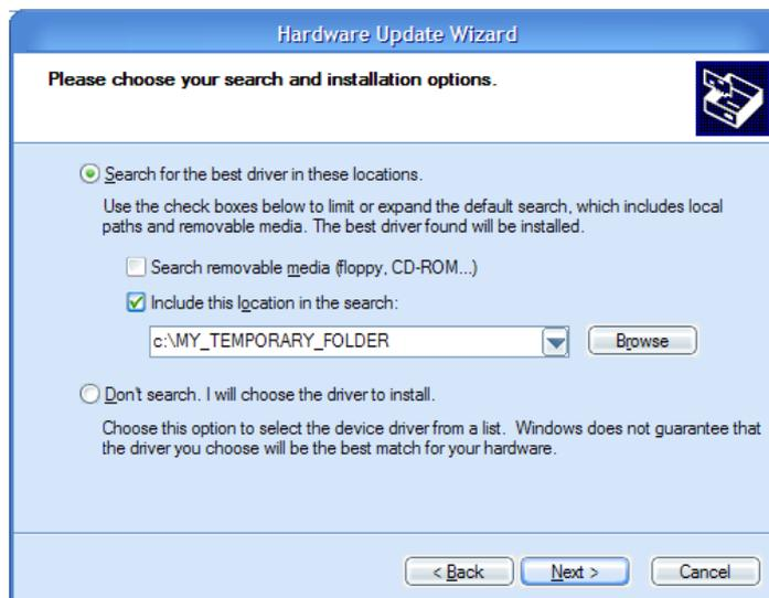
**WARNING:** The COM port number assigned by Windows to AVR-ISP500-ISO must be COM4 or below. Otherwise AvrStudio might not be able to detect the programmer. Here are the steps to change it:
