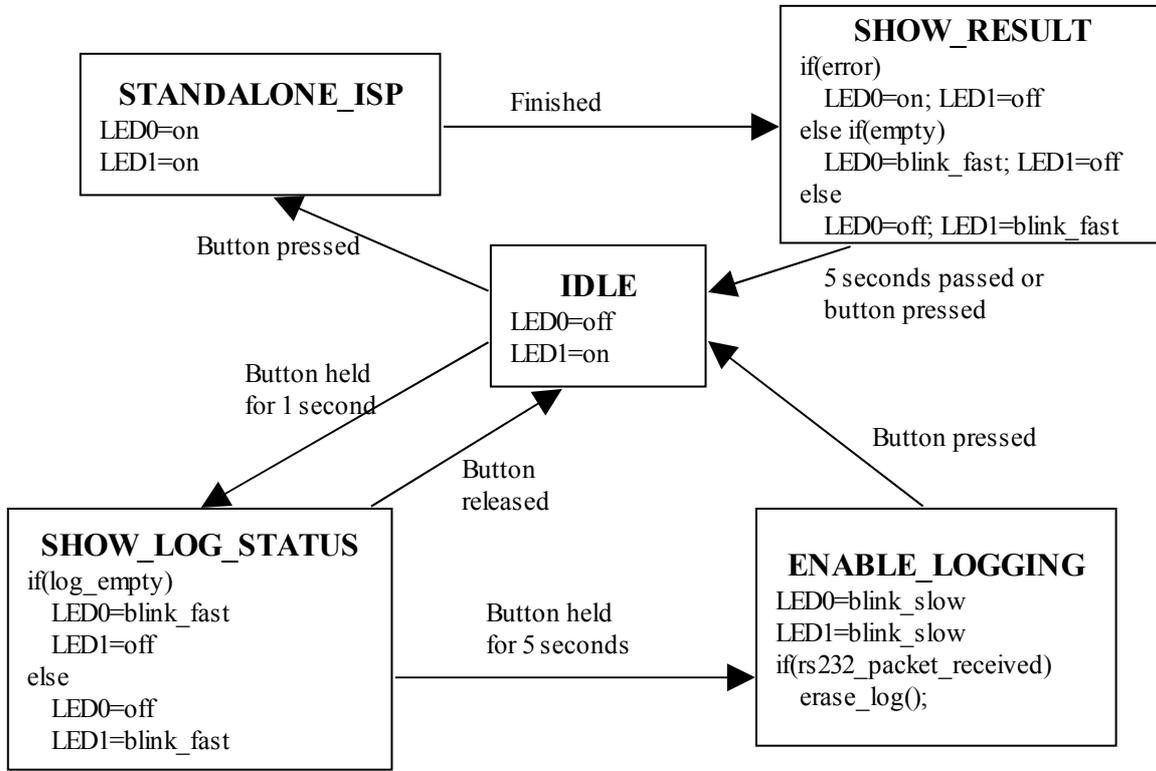
NOTE: LED0 is **RED**, and LED1 is **GREEN**. If both are on, the result is **Yellow** glow.
