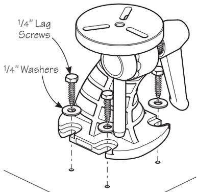
Figure 2: Carver's vise mounted using 1/4" lag screws.
