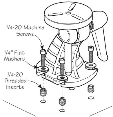
**Figure 3:** Carver's vise mounted using threaded inserts.
