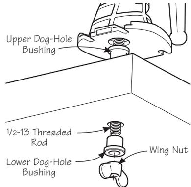
**Figure 4:** Carver's vise mounted using Veritas® Dog-Hole Mount Assembly.
