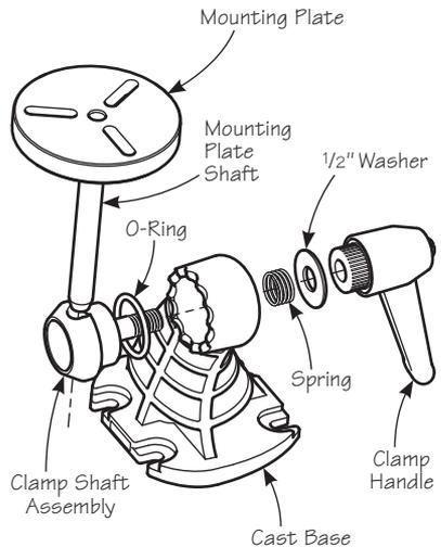
**Figure 7: Exploded assembly of the carver's vise.**
